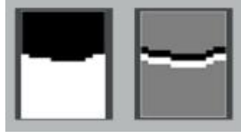
Fig. 6. The edge template (right) is derived from the boundary of the figure-ground label. The response to this template is the edge part E_{\text{dge}} in (3).
