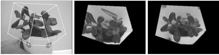
Fig. 7. Geometric errors in flower sequence. (Left) One of the original images and the outline of the quadrilateral patches. (Middle) Image generated using static texture. (Right) Image generated in the same pose using dynamic texture.
