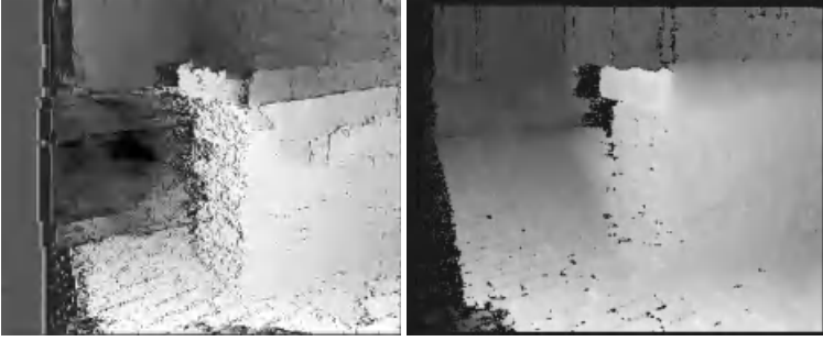
Fig. 5. Pure stereo results; Left: depth map for the dynamic path algorithm; Right: depth map for left the algorithm described in section 3, black pixels have low confidence (e.g. occlusion).
