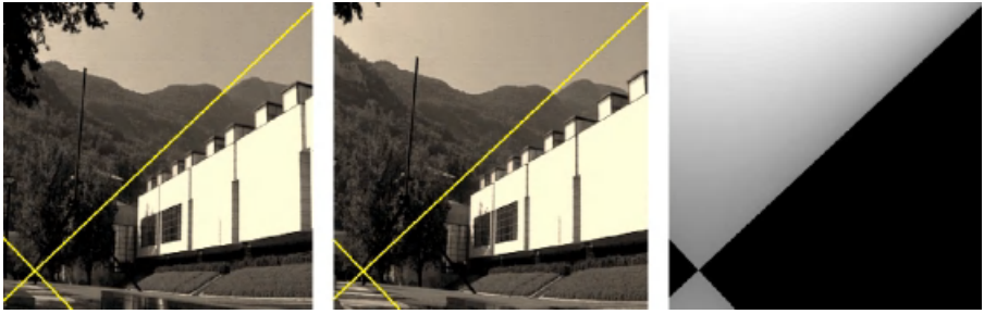
Fig. 7. A pair of images of the Grenoble museum from which one wishes to compute the focal lengths. It is assumed that the principal point \mathbf{p}_1 in the first image is the centre of the image. Shown overlaid on the first (left-hand) image are the epipolar line [\mathbf{e}_1] \times \mathbf{p}_1 and the perpendicular epipolar line [\mathbf{e}_1] \times \mathbf{I}[\mathbf{e}_1] \times \mathbf{p}_1 . Overlaid on the second (right-hand) image are the corresponding epipolar lines \mathbf{Fp}_1 and \mathbf{FI}[\mathbf{e}_1] \times \mathbf{p}_1 . From these latter two lines one may compute the focal length f_2 . Computation of the focal length f_2 will be very imprecise in this case, since the angle \theta between these two lines is close to 90^\circ , and also because one of the lines (actually \mathbf{Fp}_1 ) passes very close to the centre of the image, and hence (presumably) close to the principal point \mathbf{p}_2 . Relative accuracy of the focal length f_2 is given by (3), and is proportional to the distance of \mathbf{p}_2 from each of these two epipolar lines, and also to the tangent of the angle \theta .
