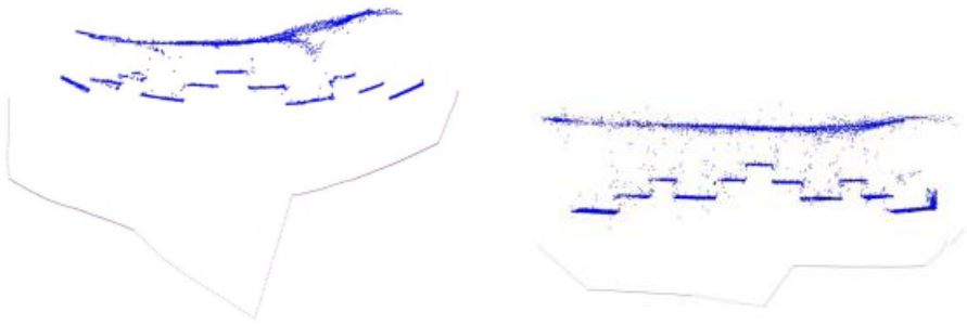
Fig. 5. Left: The recovered structure and scene when radial distortion was present but not modeled by the program. Right: The recovered structure and motion when the radial distortion was also modeled as described in this paper. The camera moved from right to left. As the system only converged after 200 frames the part of the structure on the far right still shows some residual bending.
