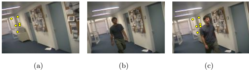
Fig. 3. Using the dual trilinear tensor to resume tracking of lost points. The images are part of a sequence of 160 images in which roughly 50 points were detected in frame 1 and tracked throughout the sequence. The points overlaid in (a) are those which were lost as some point due to the passing person (b) and recovered in (c).
