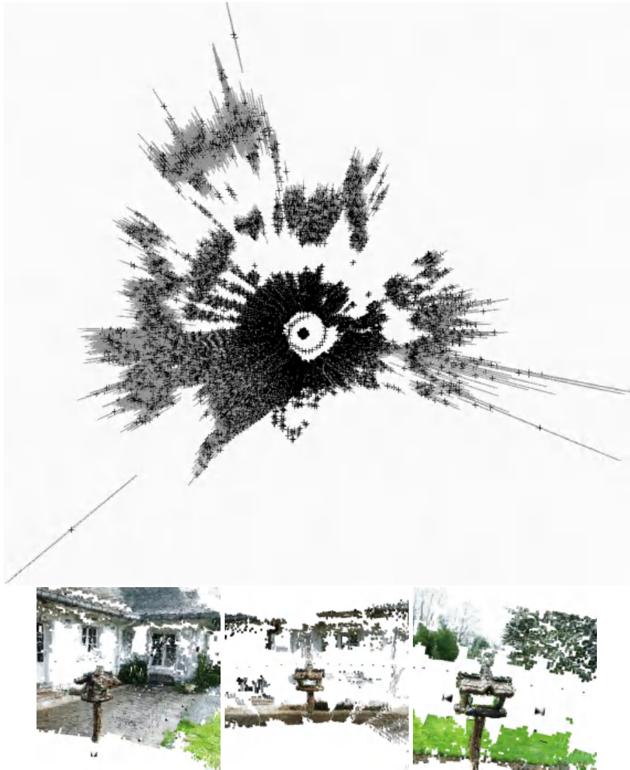
Fig. 7. Top view of the 90% confidence ellipsoids and 3 re-projected views of QUASI reconstruction. The small square shaped connected component at the center is the reconstructed bird cage while the visible crosses forming a circle are camera positions.
