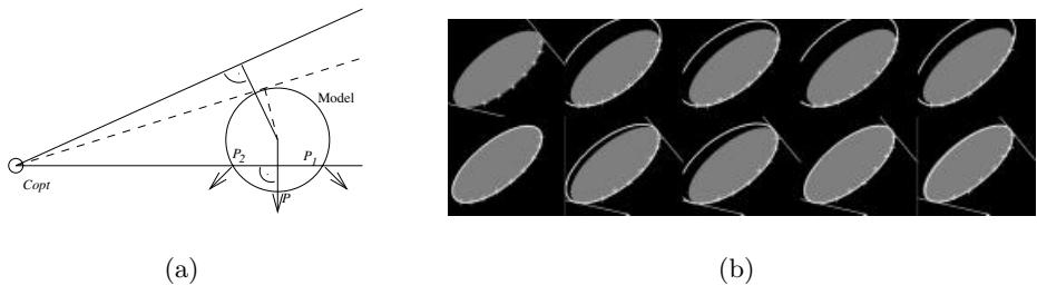
Fig. 2. Silhouette constraints. (a) Two lines of sight going through the camera optical center. In both cases, at the point that minimizes F along the line, the gradient of F is perpendicular to the line. But only in the case of the dashed line that is actually tangent to the surface, is this point on the surface and thus satisfies both criteria of Section 3.2. (b) The top row depicts the results of fitting an ellipse to slightly noisy 2-D points, shown as white crosses. The computed ellipses are much too large. The bottom row depicts the fit to the same points, but under the constraint that the ellipse be tangent to the white lines. The results are much improved.
