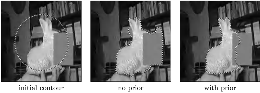
Fig. 9. Begin of the tracking sequence: initial contour, segmentation without prior, segmentation upon introducing the nonlinear prior on the contour.
